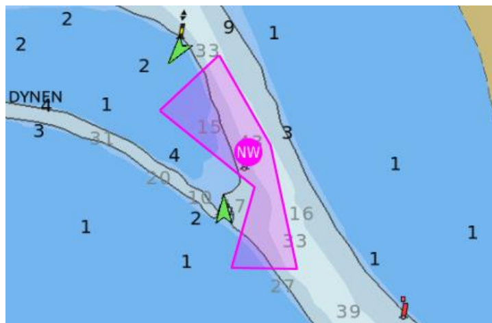
Figure 1: Snippet of an ECDIS showing AIS data (other ships as green icons) and AIS 2.0 information (navigational warning with a polygon-shaped area)
